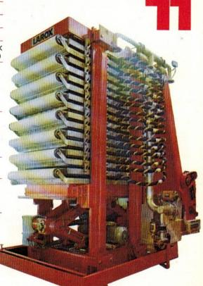
A single filter unit, forming a filter chamber, consists of the plate, frame, collector sections, diaphragm, supporting grid and perforated sheet.
